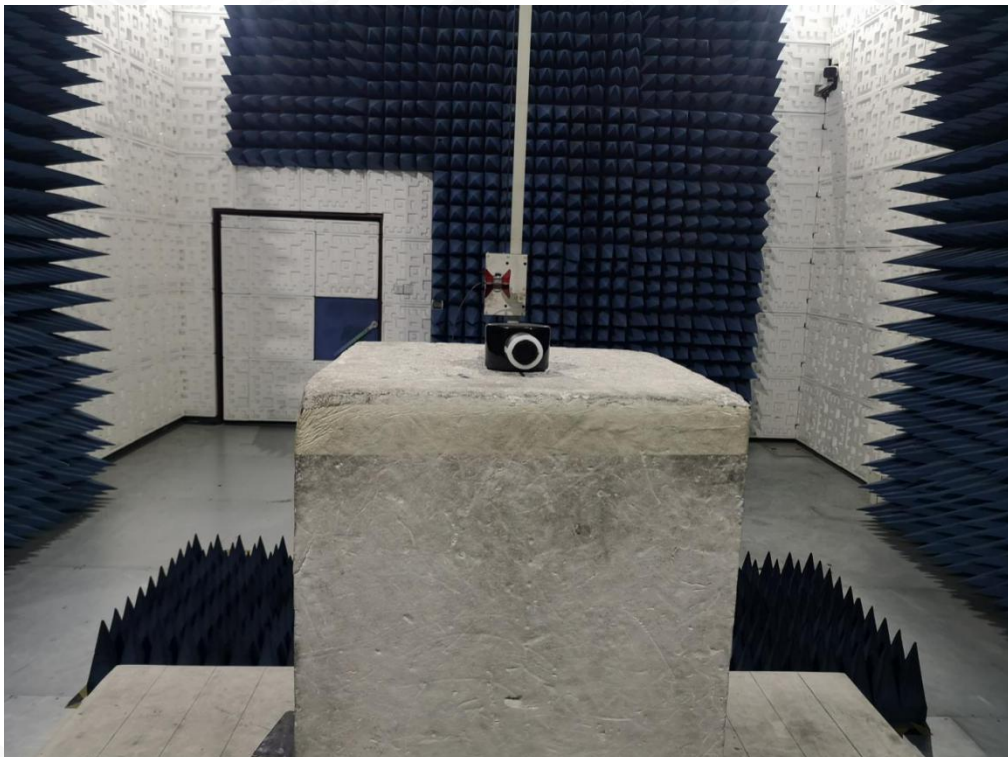
RADIATED EMISSION TEST SETUP ABOVE 1GHZ
