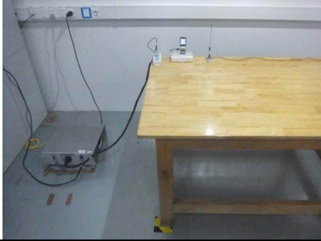
Conducted Emissions Test Setup Front View
