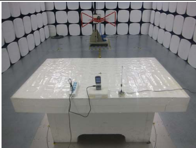
Conducted Emissions Test Setup Front View
