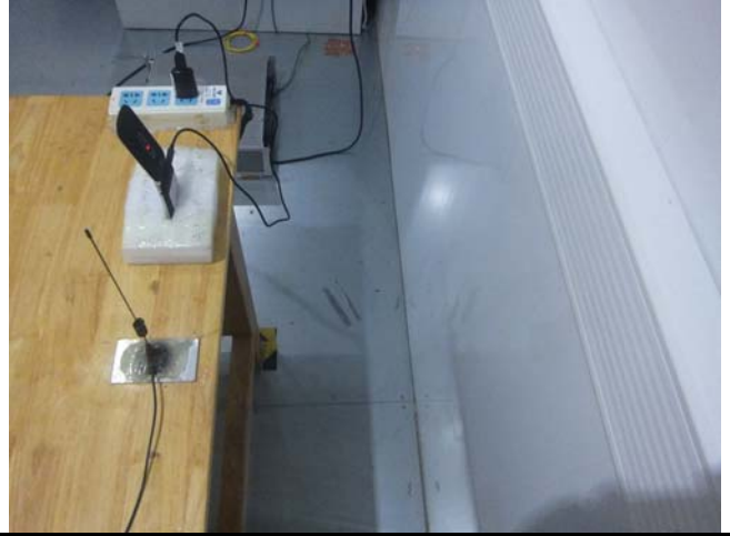
Conducted Emissions Test Setup Side View
