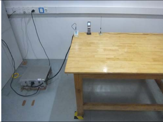
Conducted Emissions Test Setup Front View
