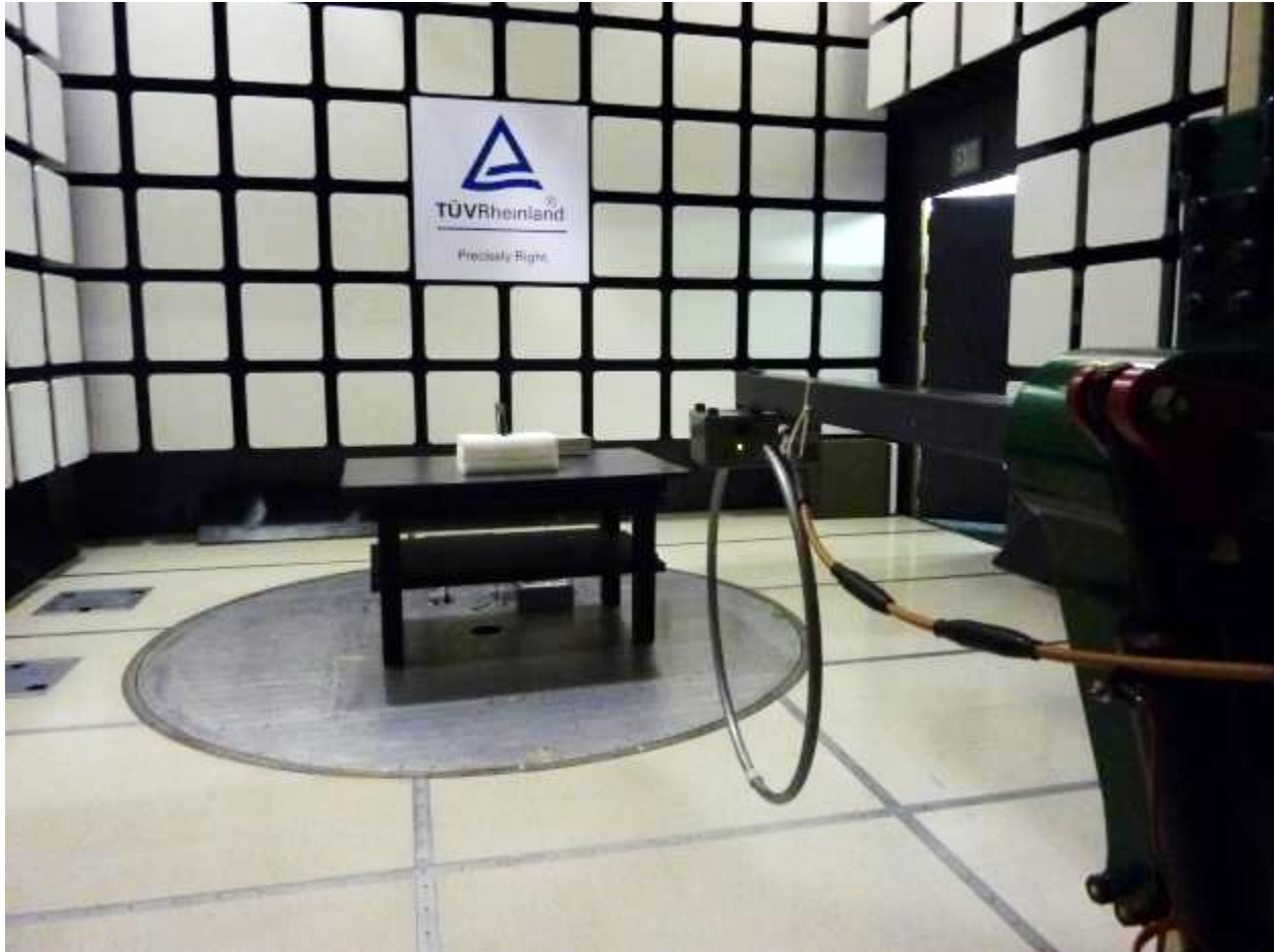
Figure 3 – Radiated Emissions 9 kHz to 30 MHz Antenna Facing EUT 90 Degrees
