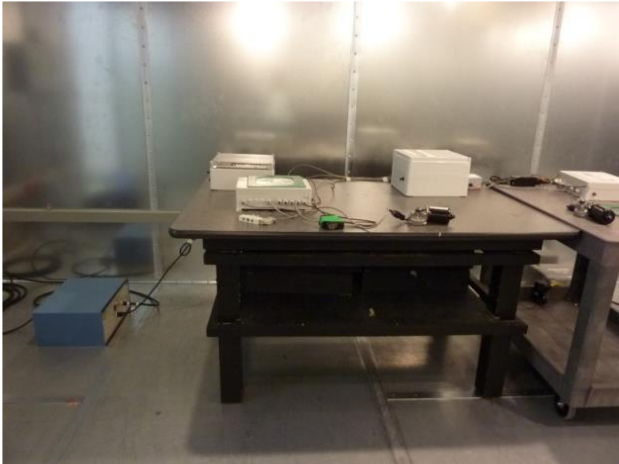
Figure 8 – AC Line Conducted Emissions
