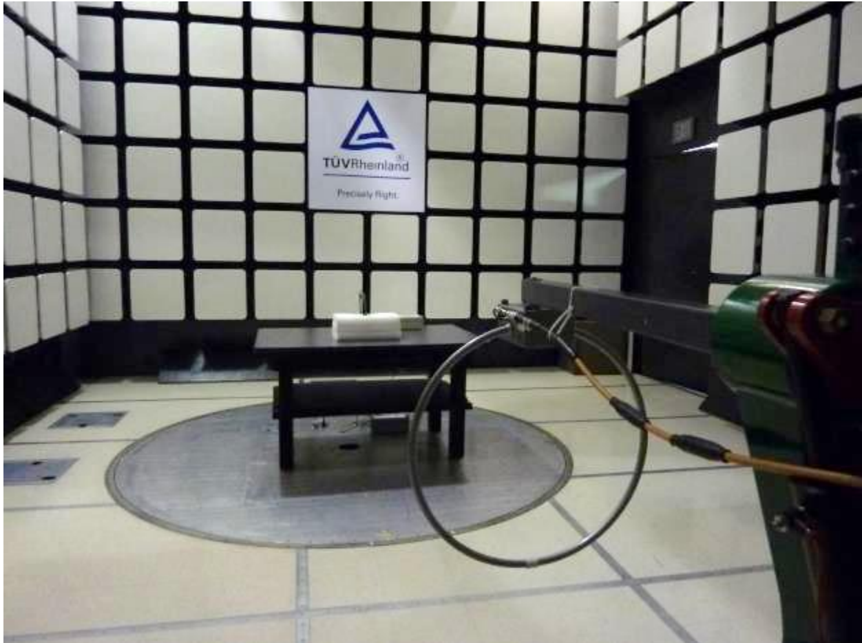
Figure 1 – Radiated Emissions 9 kHz to 30 MHz Antenna Facing EUT 0 Degrees
