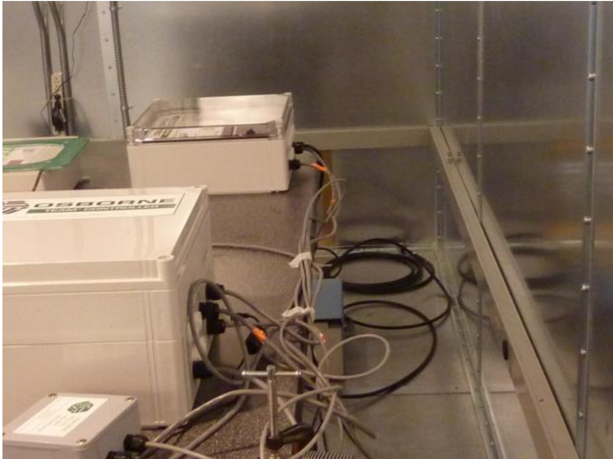
Figure 9 – AC Line Conducted Emissions
