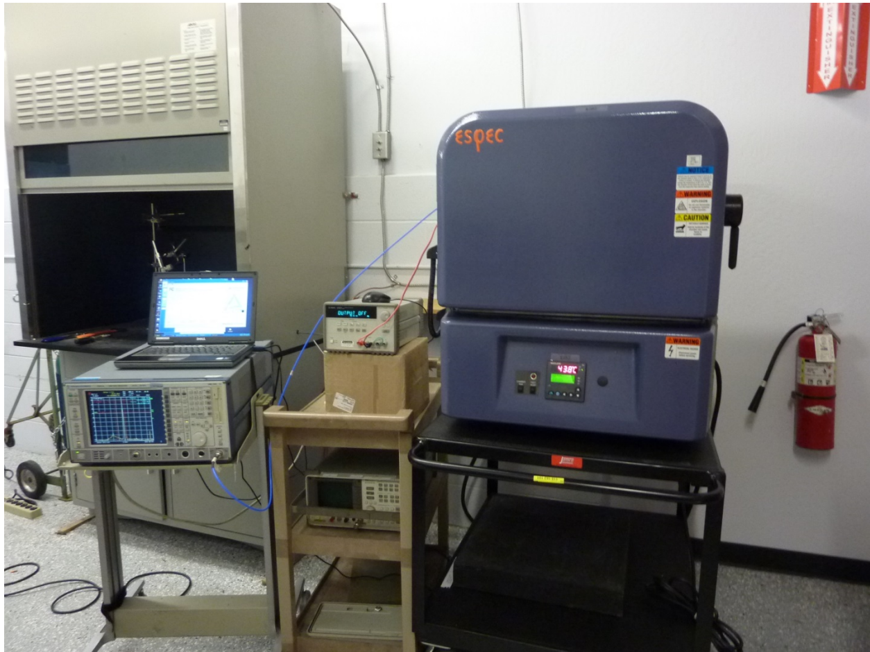
Figure 7 – Conducted and temperature test setup
