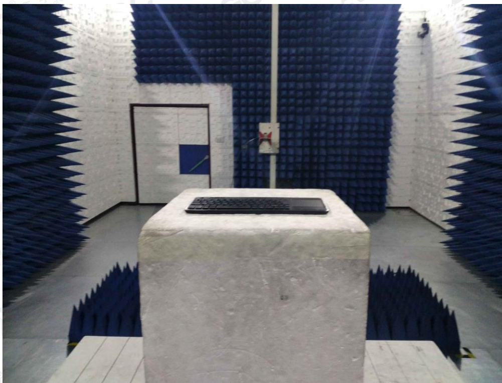
FCC RADIATED EMISSION TEST SETUP ABOVE 1GHZ
