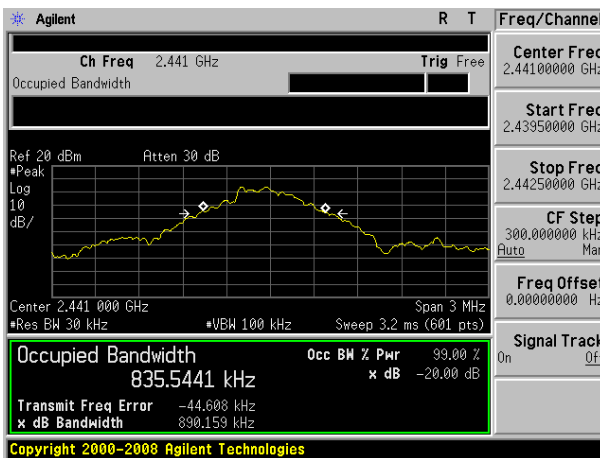
20dB Bandwidth plot on channel 39 (1Mbps)
