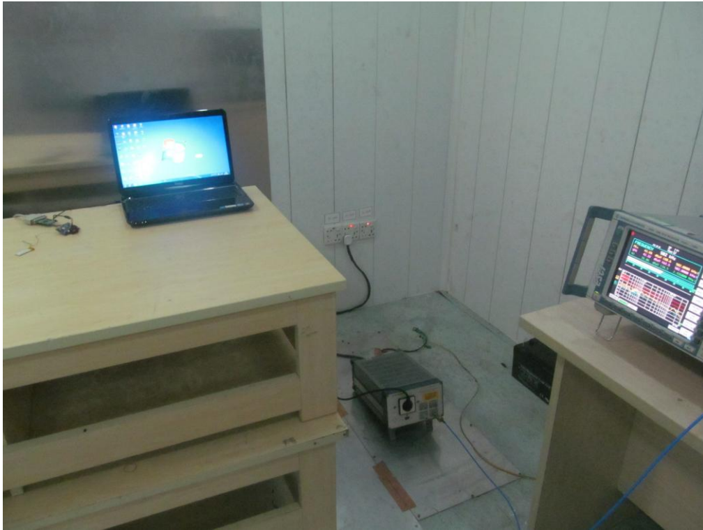
FCC RADIATED EMISSION TEST SETUP
