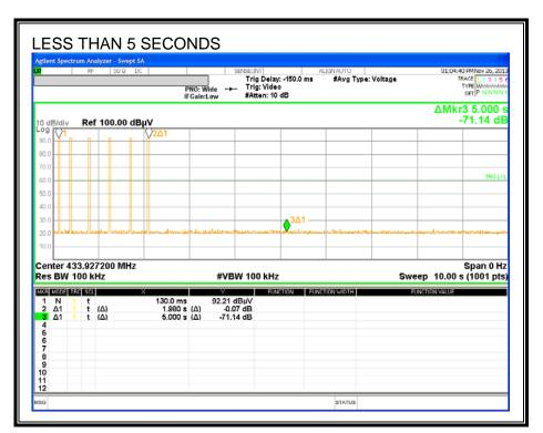
The above represents a magnet moved quickly towards the EUT. (e.g., closing a window.)
