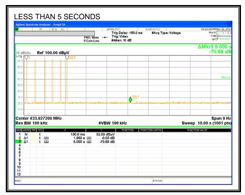
The above represents a magnet moved quickly away from the EUT. (e.g., opening a window.)
