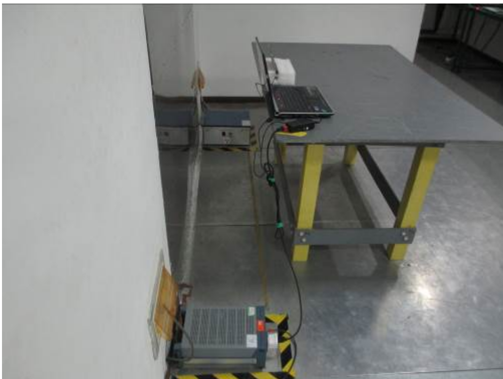
Conducted Emissions Test Setup Side View
