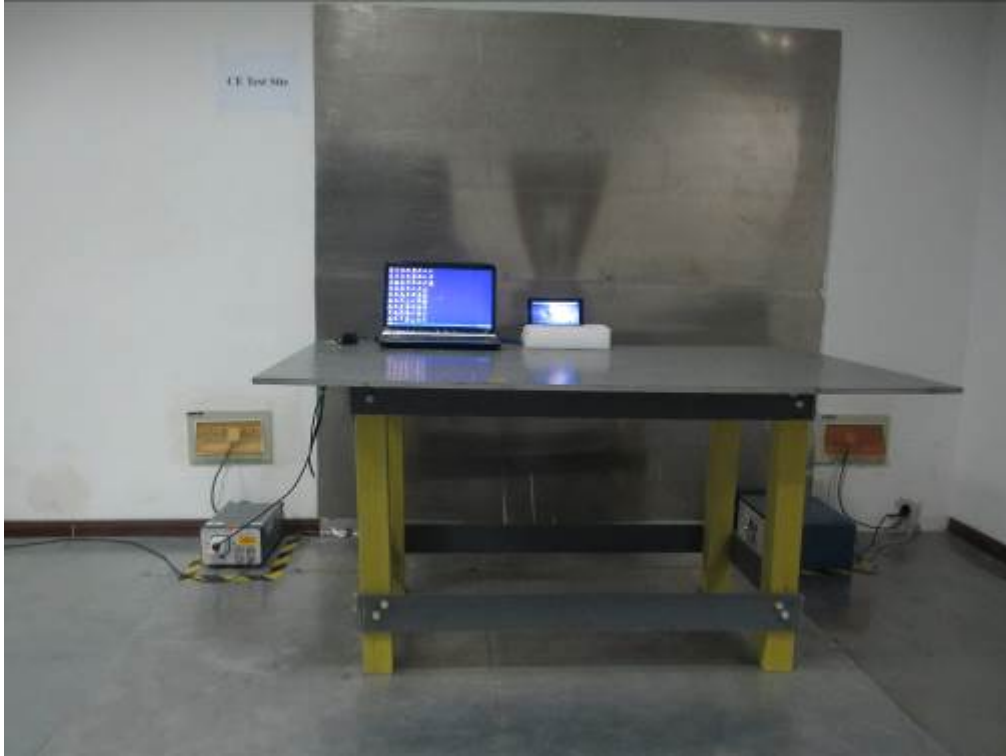
Conducted Emissions Test Setup Front View
