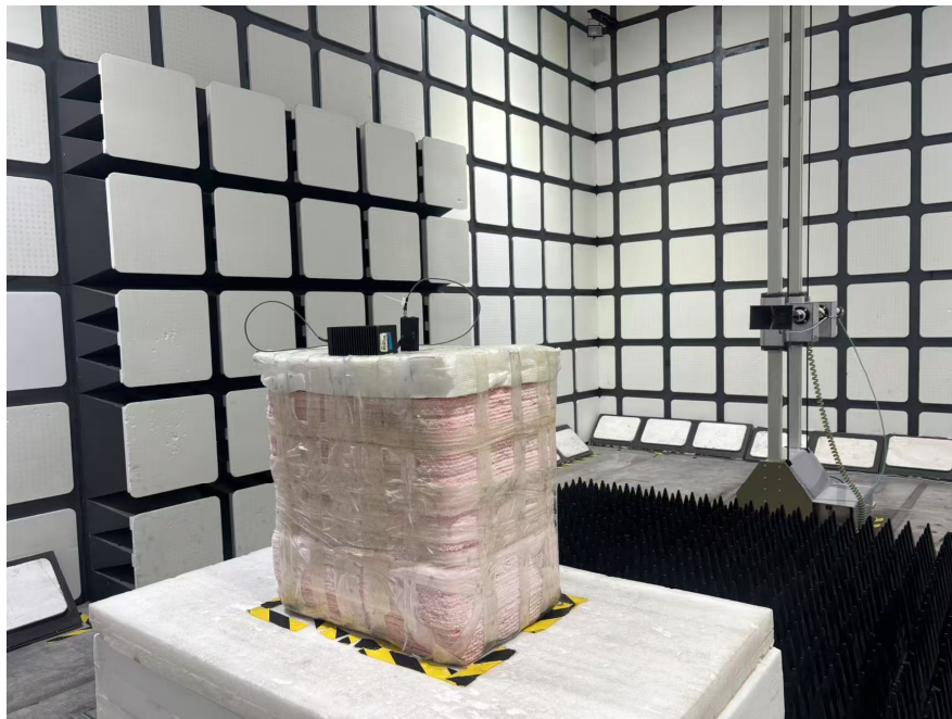
Radiated Emissions View (Above 1 GHz)
