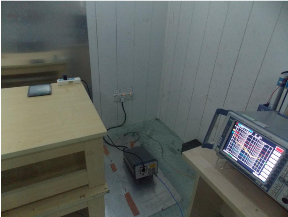
FCC RADIATED EMISSION TEST SETUP
