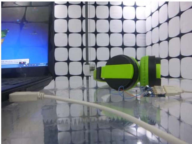
Radiated Spurious Emissions Test Above 1GHz
