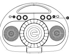
Connect microphone(s) as shown on page 4, and slide the ON/OFF switch to the ON position.
