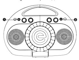
Insert a microphone's plug into the Mic 1 jack 1. Insert the other microphone's plug into the Mic 2 jack 2 (if desired).
