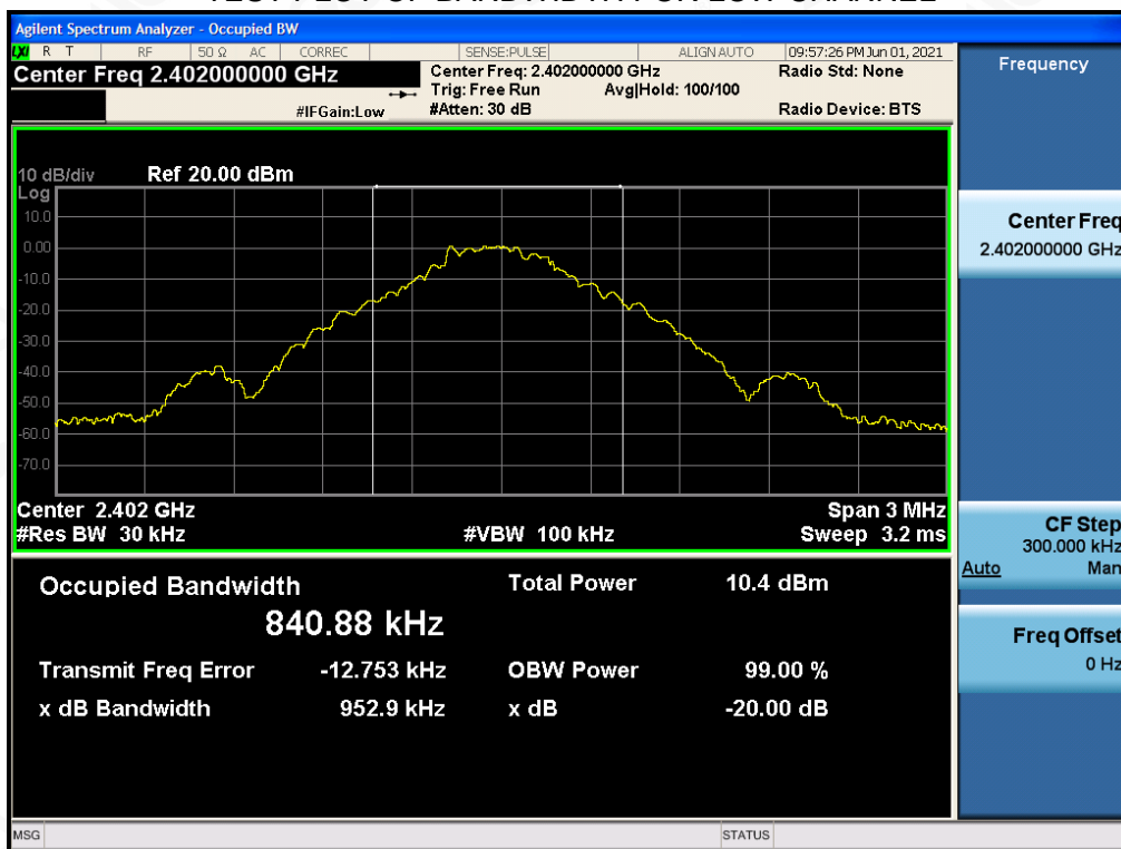
TEST PLOT OF BANDWIDTH FOR LOW CHANNEL
