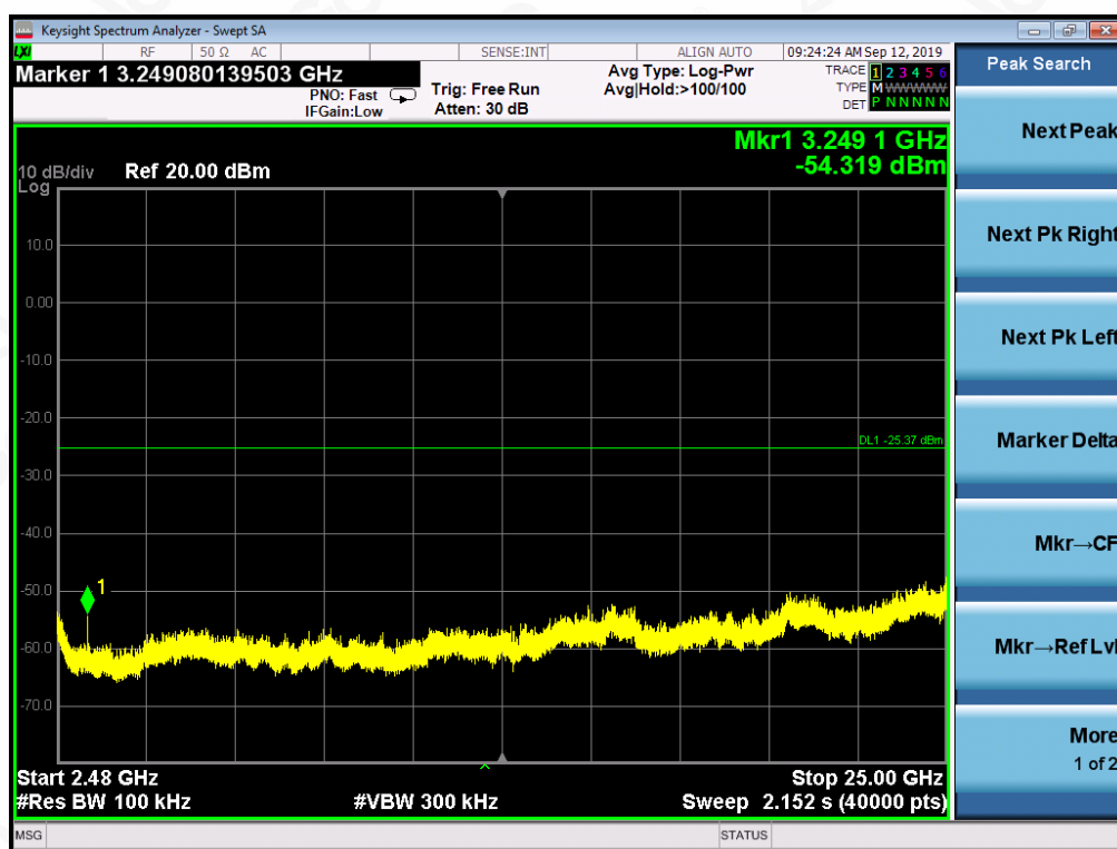
TEST PLOT OF OUT OF BAND EMISSIONS THE WORST CASE OF (802.11g with data rate 6) FOR MODULATION IN HIGH CHANNEL
