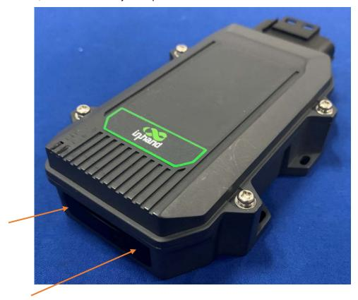
Arrow position for SIM card cover. Open the cover and insert the SIM card according to the SIM card direction indicated on the cover.
