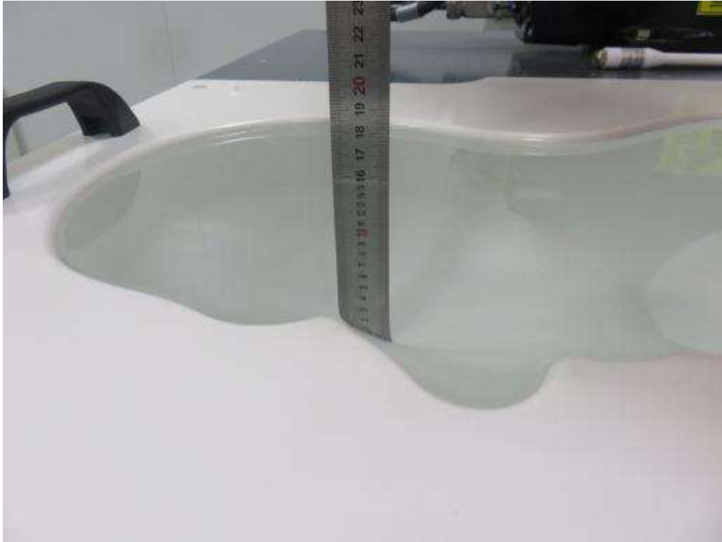
Photograph of the depth in the Body Phantom( \geq 15 cm)
