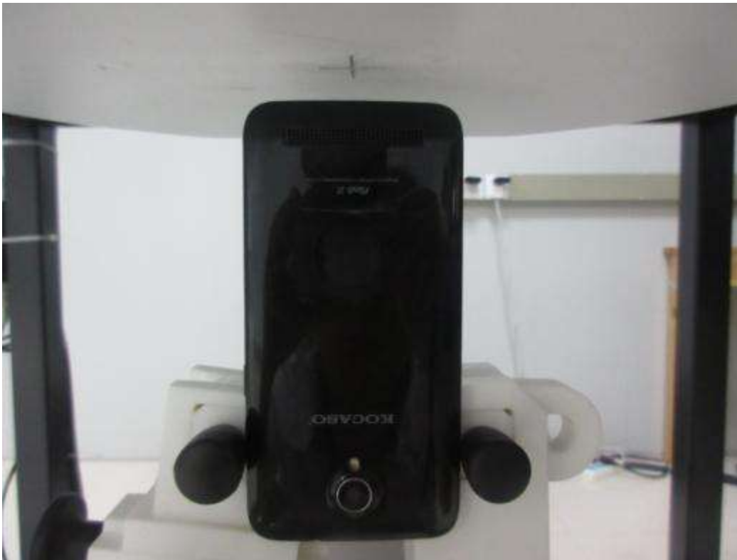
10mm body-worn Bottom Side Setup Photo(hotspot)
