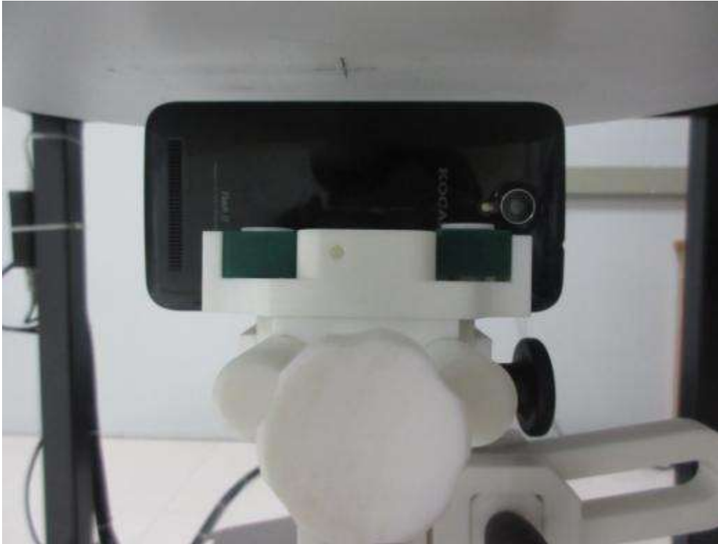
10mm body-worn Right Side Setup Photo(hotspot)
