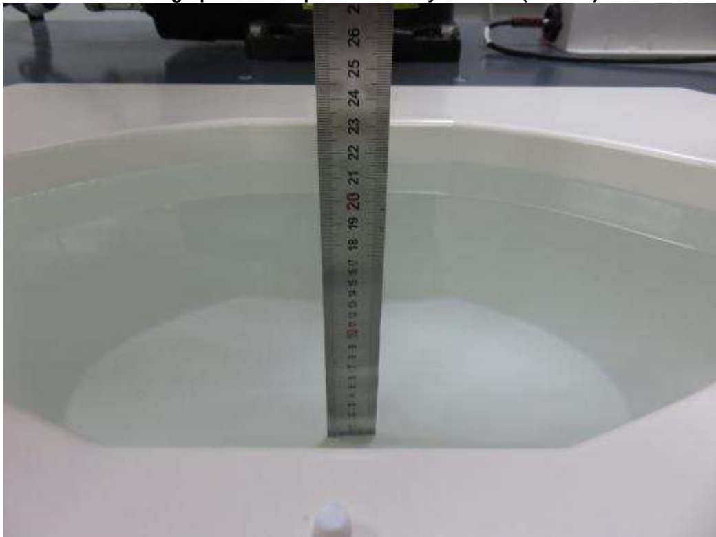
Photograph of the depth in the Body Phantom( \geq 15 cm)
