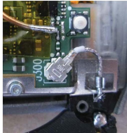
Coax cable feed to monopole antenna molded into the watch band.
