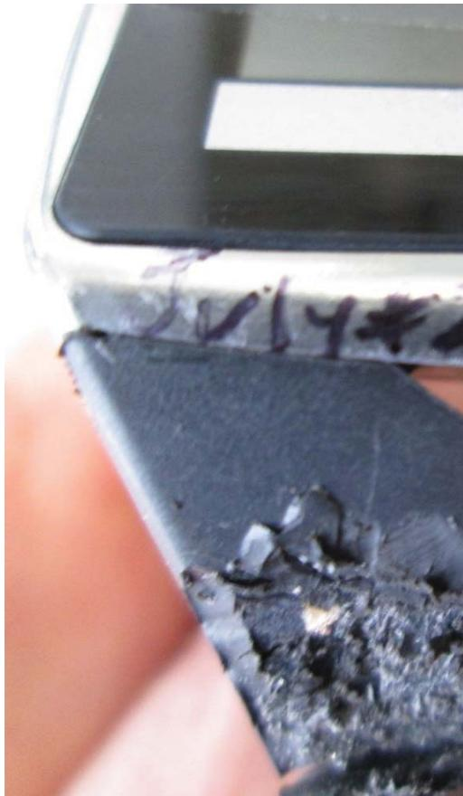
The antenna is a monopole molded into the watch band. This photo shows the rubber cut away to expose the end of the antenna.
