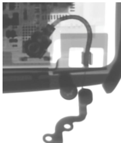
X-Ray shows coax feed and antenna element molded into watch band.
