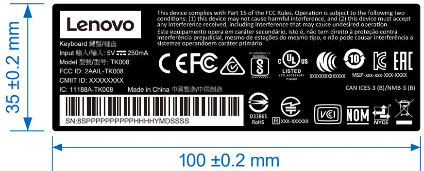
1. Size: 100mm (L) x 35mm (W) , Tolerance: ±0.2mm
