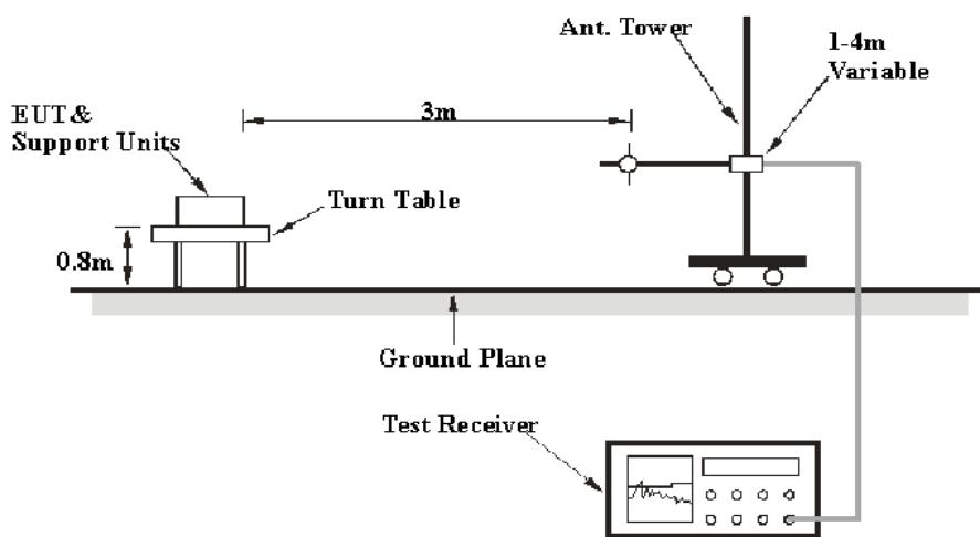
The radiated emission tests were performed in the 3 meters chamber test site, using the setup accordance with the ANSI C63.4-2003. The specification used was the FCC Part 15.109, Class B limits.
