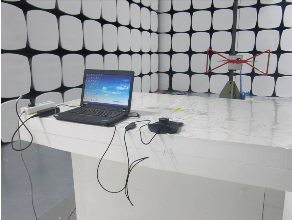
Radiated Spurious Emissions Test Setup Below 1GHz - Front View (3Dconnexion USB HUB(Model:3DX-600049) has been tested)
