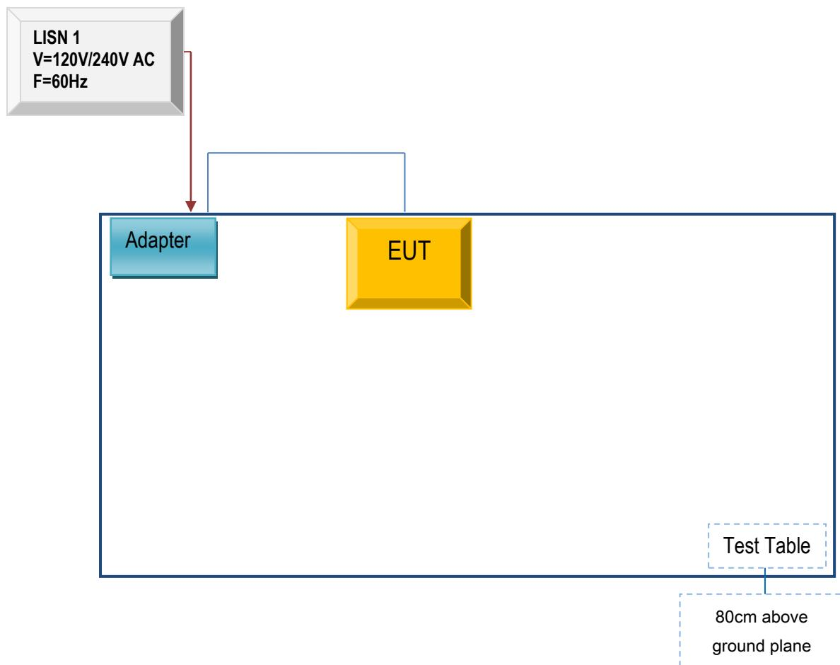
Block Configuration Diagram for Radiated Emissions ( Below 1GHz ) .
