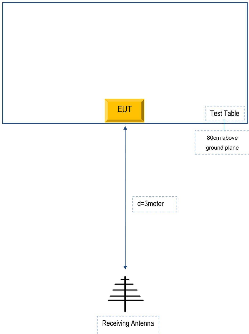
Block Configuration Diagram for Radiated Emissions ( Above 1GHz ) .
