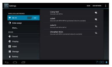
b. WIFI setting and network connecting: Click "Wi-Fi setting" to enter and the system will automatically find WIFI network name.
