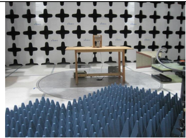
Test setup at 3 meter distance (>1GHz) - Front
