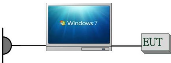
Fig. 2-1 Radiated Emission Configuration
