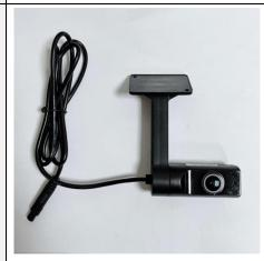
Use its own 3M adhesive installed in the rear-view mirror above the main driver's side (if the DSM use the camera for algorithm detection, you can slightly tilt the lens to the direction of the main driver about 10 degrees, so that the main driver's face can be completely in the lens screen)
