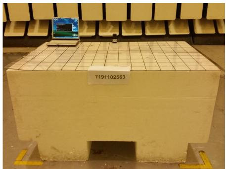
Radiated Emissions Test Setup (Front View)
