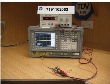
**Band Edge Compliance (Conducted) Test Setup**
