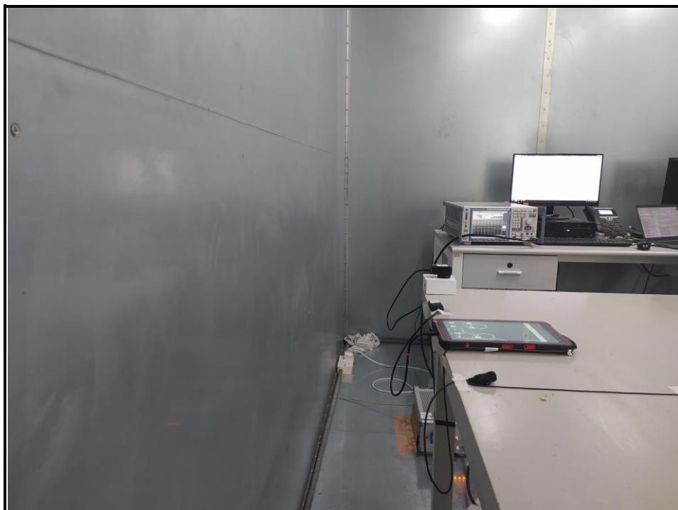
Fig. 3 Power line conducted emission setup photo
