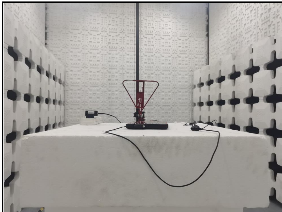
Fig. 1 Radiated emission setup photo(Below 30MHz)
