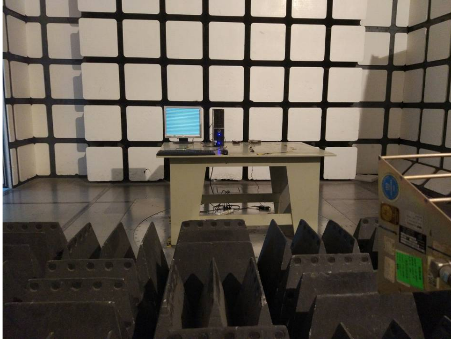
Radiated Emissions – Front View (Above 1 GHz)
