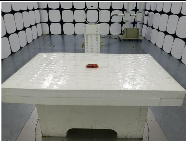
Radiated Emissions Test Setup 1MHz-30MHz
