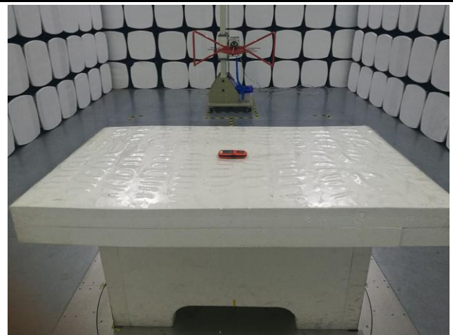
Radiated Emissions Test Setup 30MHz-1GHz
