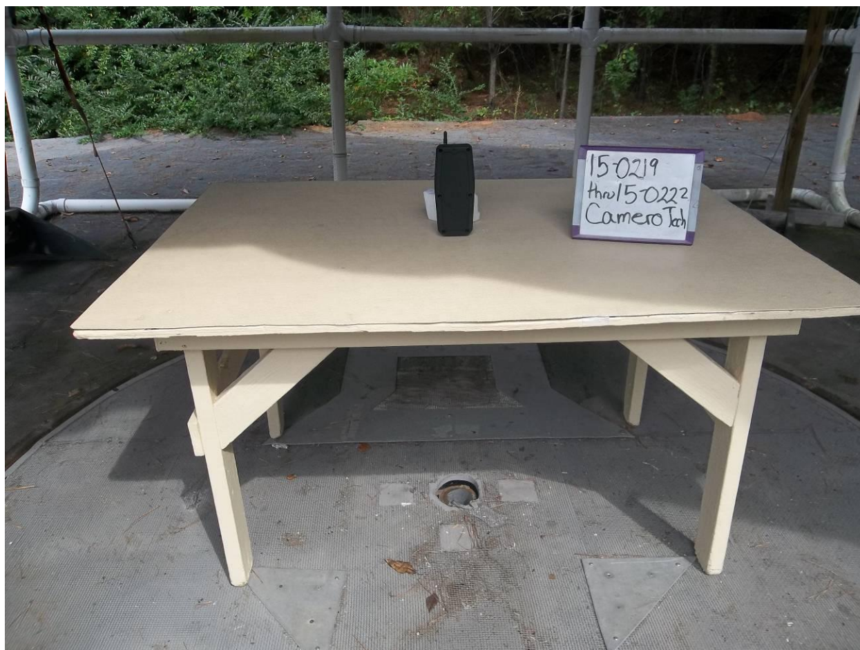
Figure 1. Radiated Emissions Test Setup Below 1 GHz, Front
