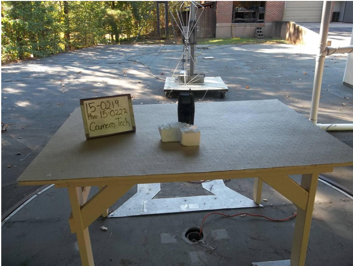
Figure 5. Radiated Emissions Test Setup, 30 MHz to 200 MHz, Back
