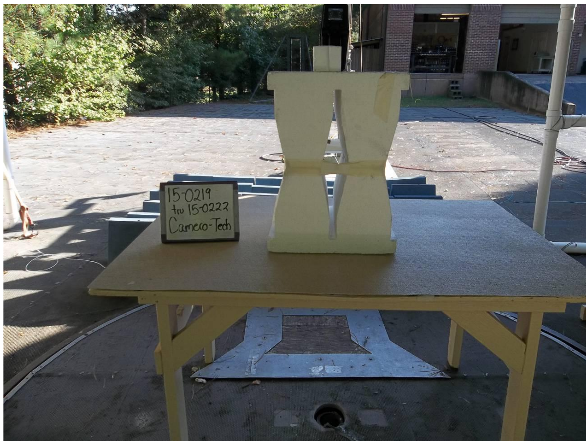
Figure 7. Radiated Emission Test Setup, above 1 GHz, Back
