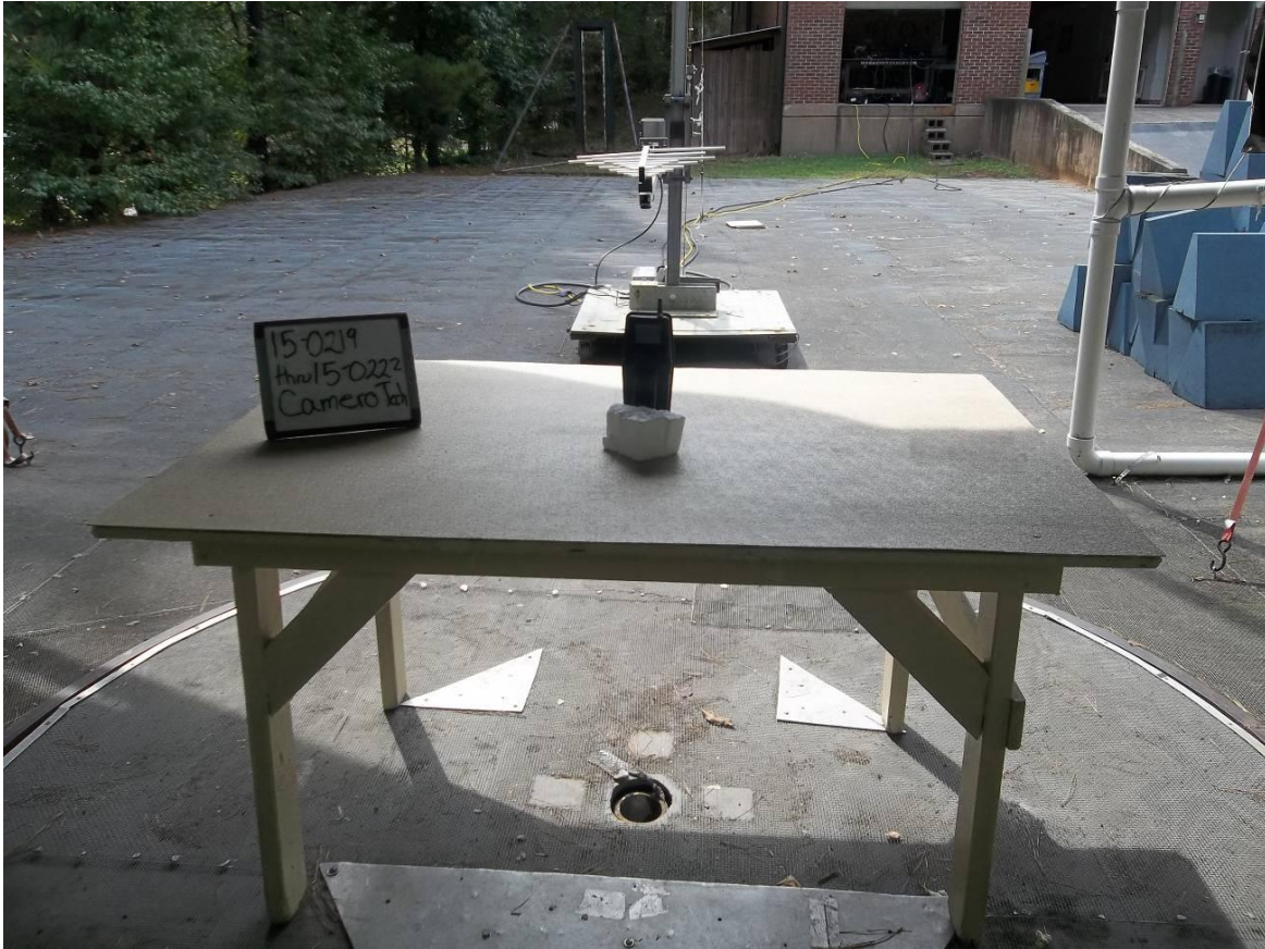
Figure 6. Radiated Emissions Test Setup, 200 MHz to 1GHz, Back
