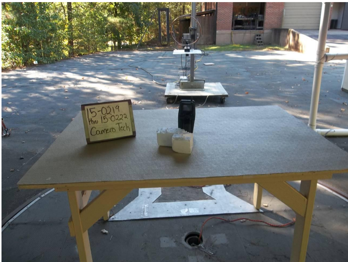
Figure 4. Radiated Emissions Test Setup, 9 kHz to 30 MHz, Back
