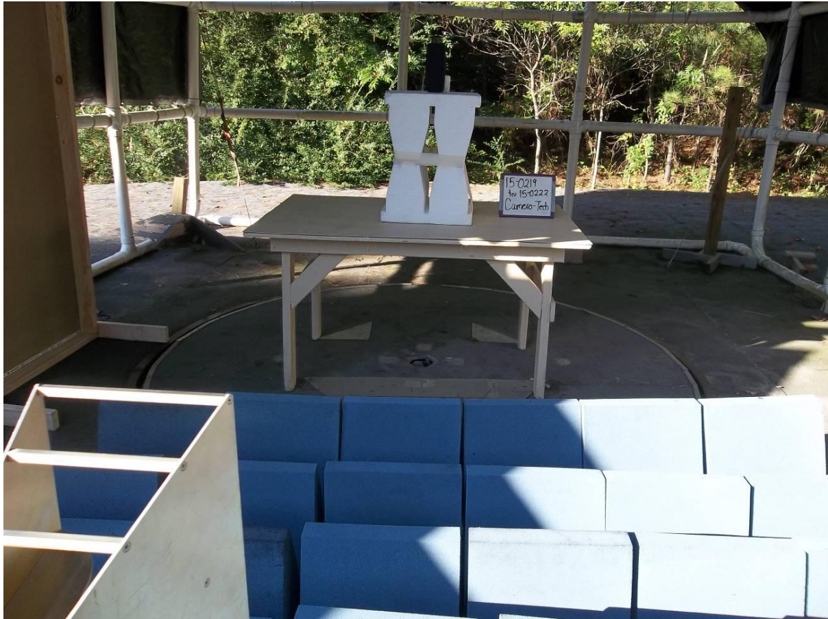
Figure 2. Radiated Emissions Test Setup Above 1 GHz, Zigbee Radio, Front
