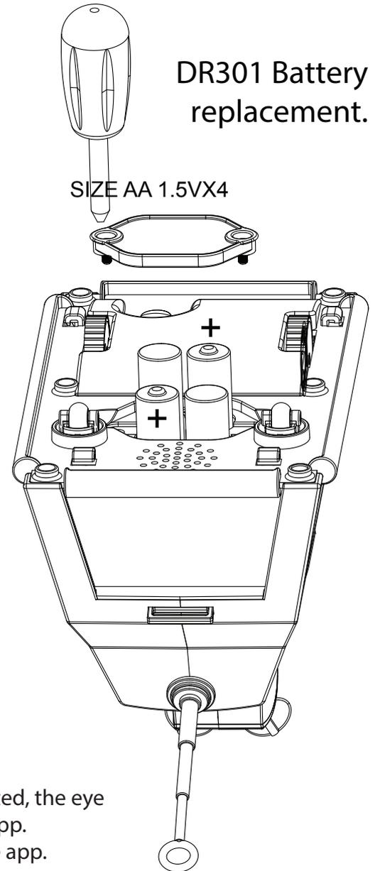
Under the environment with electrostatic discharge, the product may malfunction. It requires user to reset the unit by replacing the batteries.
