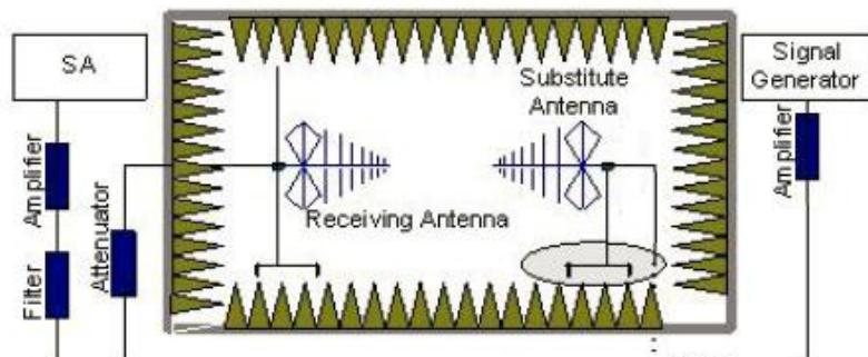
In the chamber, a substitution antenna for the frequency band of interest is placed at the reference point of the chamber. An RF Signal source for the frequency band of interest is connected to the substitution antenna with a cable that has been constructed to not interfere with
