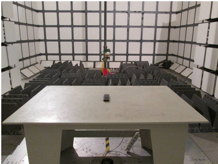
Radiated Emissions View (Above 1 GHz)
