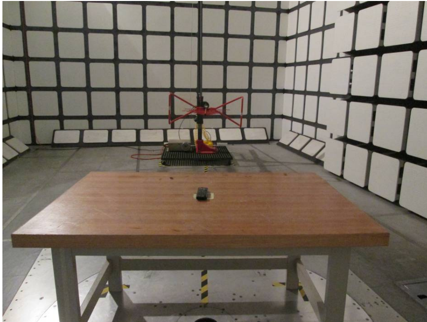
Radiated Emissions View (Below 1 GHz)
