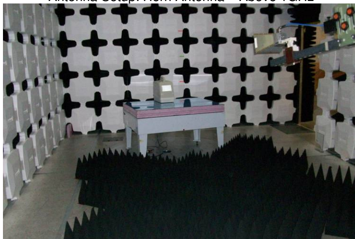
Antenna Setup: Horn Antenna – Above 1GHz
