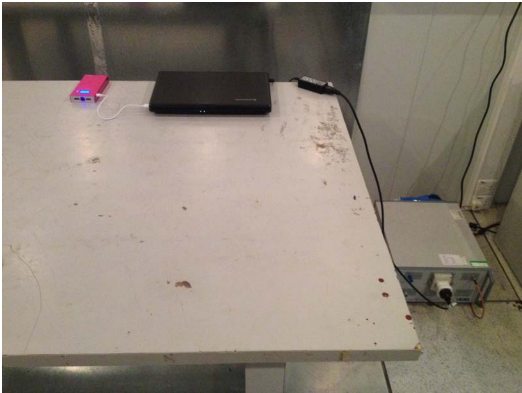
Conducted Emission test view
