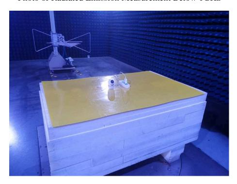
Photo of Radiated Emission Measurement Above 1GHz
