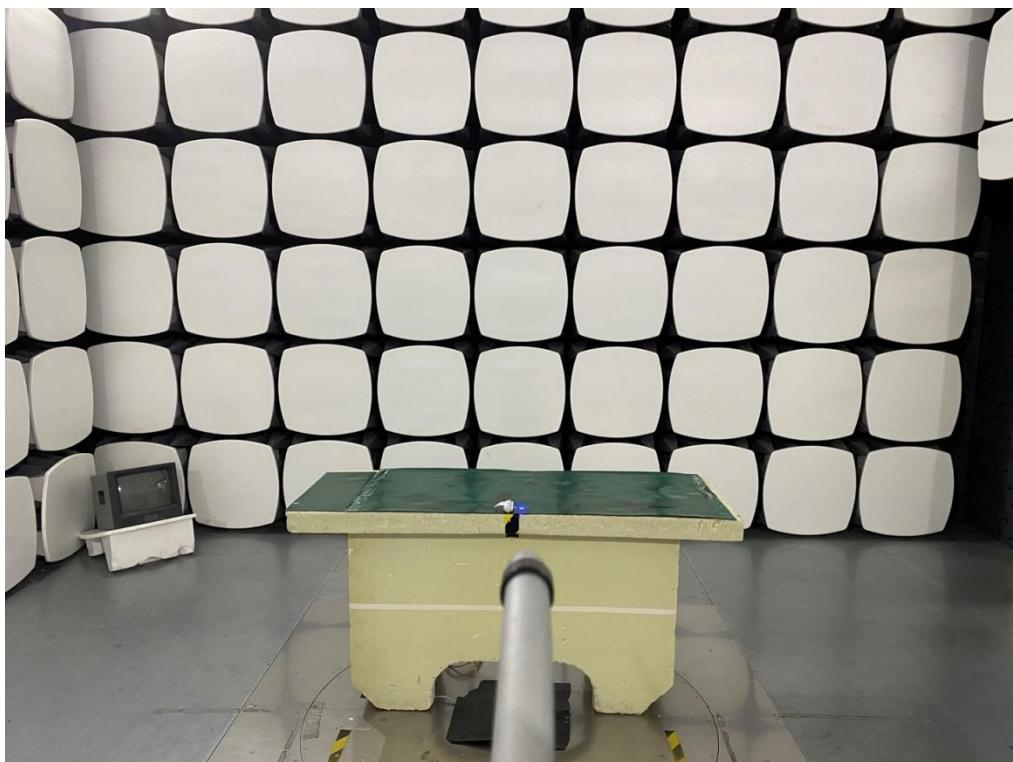
**Radiated Emissions Test Photos****30 MHz to 1000 MHz**
