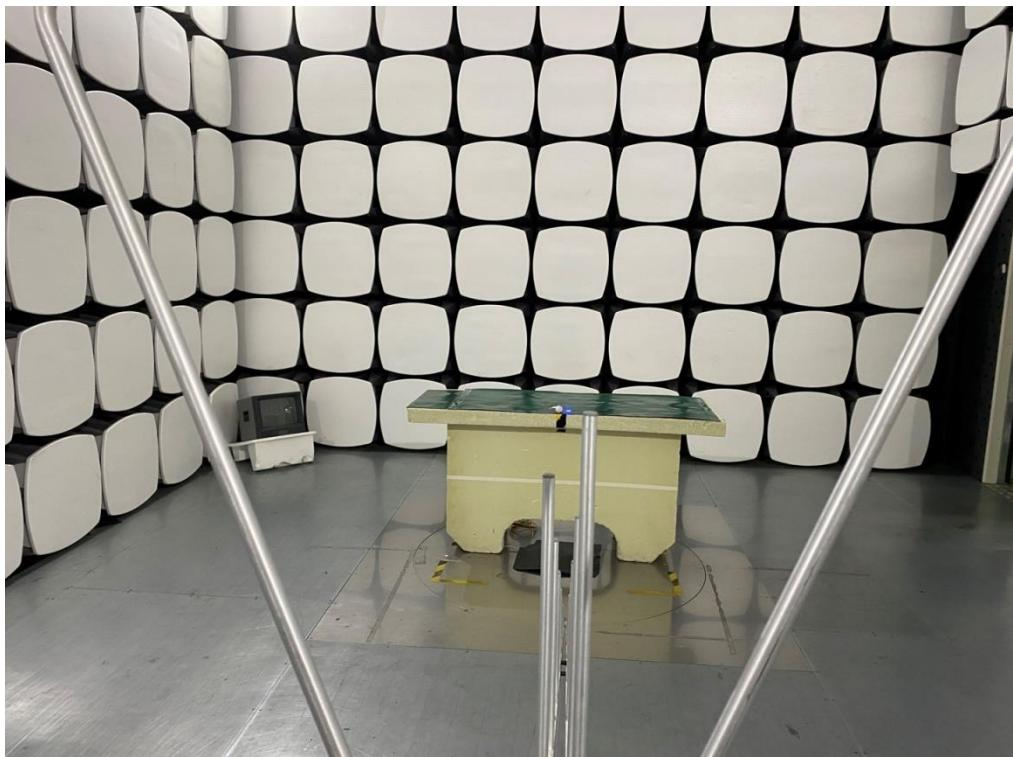
**Radiated Emissions Test Photos****Above 1 GHz**
