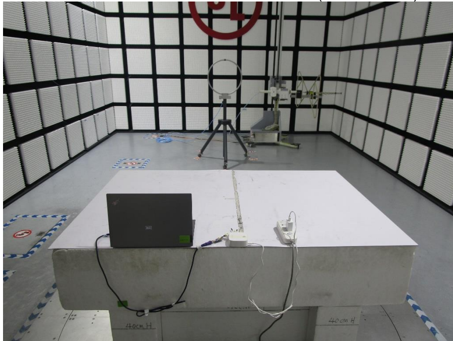
RADIATED RF MEASUREMENT SETUP (Below 30MHz)
