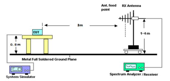
For radiated test from above 1GHz
