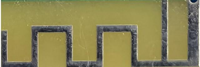
A photograph showing a close-up view of a printed circuit board (PCB) antenna. The antenna is a compact, rectangular structure with a gold-colored finish. It features a central vertical element and two horizontal arms extending from the sides, each ending in a small square cutout. The overall dimensions are 14mm in width and 5mm in height.
