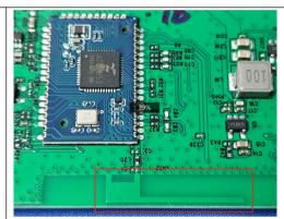
The antenna is PCB antenna.
