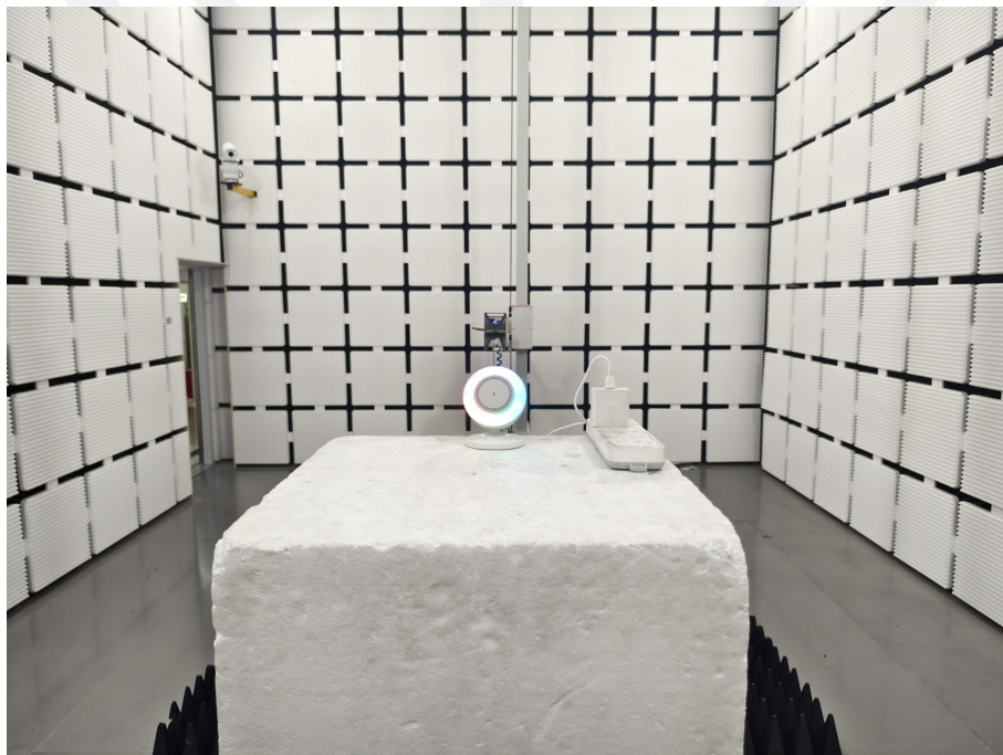
Spurious Radiation Emissions Test (> 1G)
