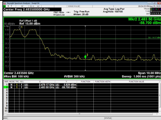
Out Of Band Emission(Right) GFSK_DH5_Channel Hopping
