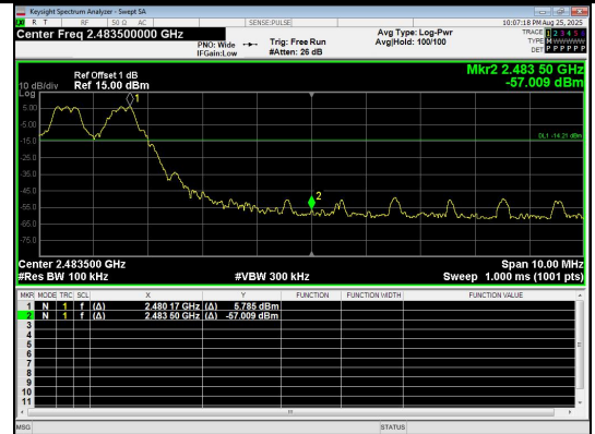
Out Of Band Emission(Right) \pi/4 DQPSK_2-DH5_Channel Hopping
