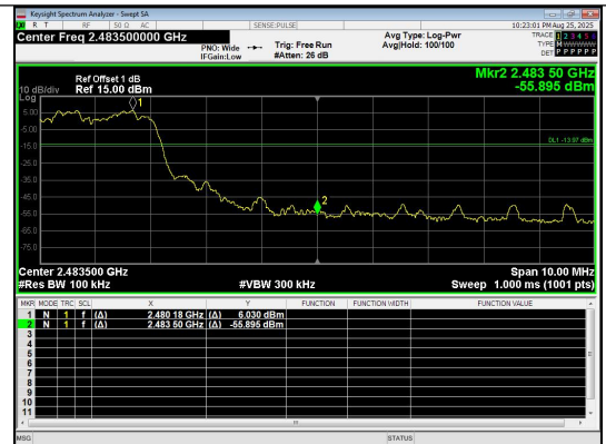
Out Of Band Emission(Right) 8DPSK_3-DH5_Channel Hopping
