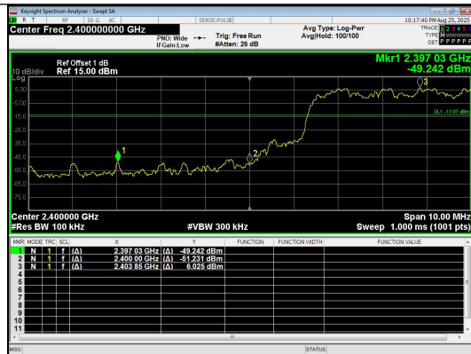
Out Of Band Emission(Left) 8DPSK_3-DH5_Channel Hopping
