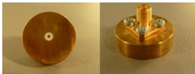
Figure 1 – MVG LIMESAR Dielectric Probe
