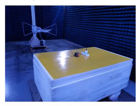
Radiated Spurious Emissions Test View (Blow 30MHz)
