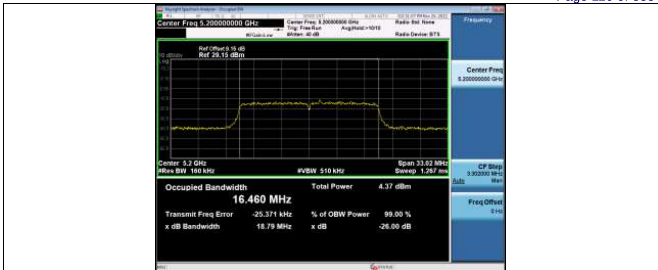
-26dB and 99% Emission Bandwidth 5_2GWiFi_NVNT_ANT5_802_11a_5240_20M
