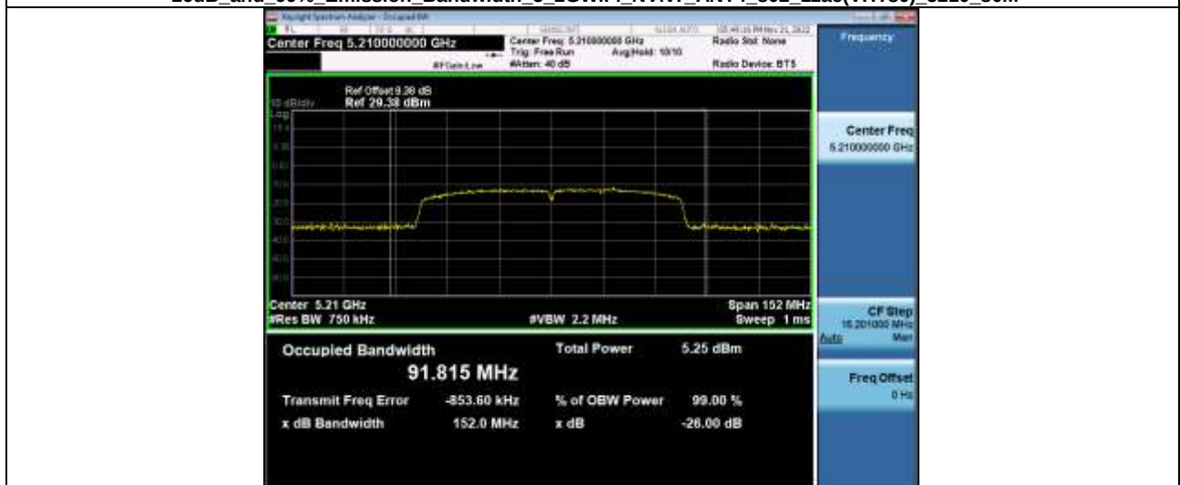
-26dB and 99% Emission Bandwidth 5_2GWiFi_NVNT_ANT4_802_11ac(VHT80)_5210_80M
