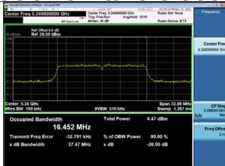
-26dB and 99% Emission Bandwidth 5_2GWiFi_NVNT_ANT1_802_11a_5240_20M
