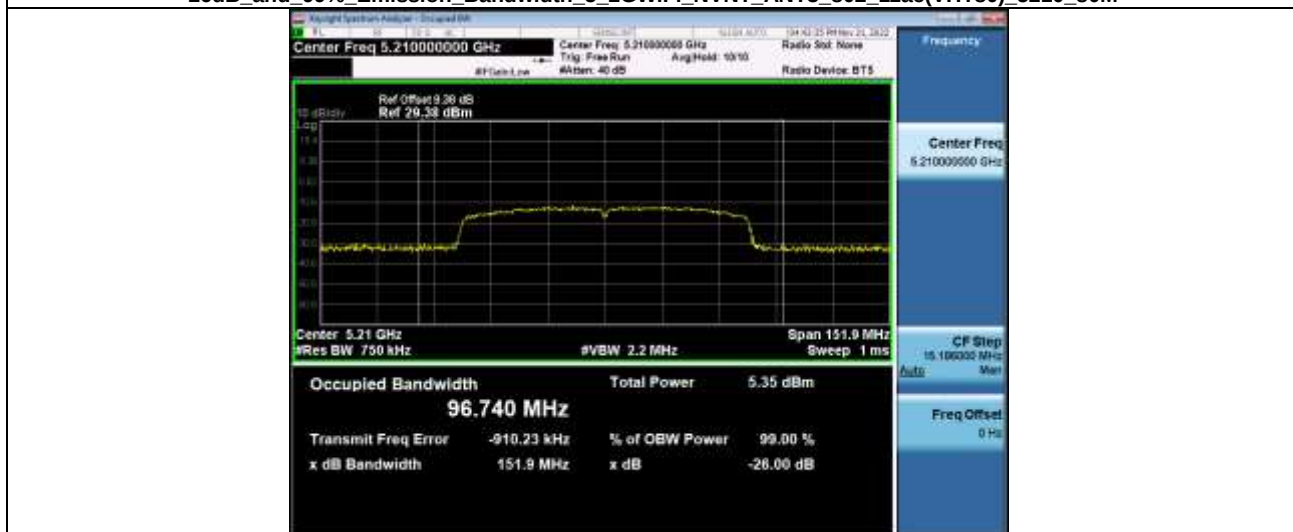
-26dB and 99% Emission Bandwidth 5_2GWiFi_NVNT_ANT3_802_11ac(VHT80)_5210_80M
