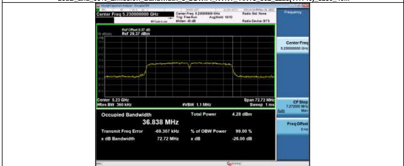
-26dB and 99% Emission Bandwidth 5_2GWiFi_NVNT_ANT5_802_11ac(VHT80)_5210_80M
