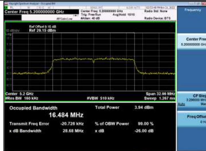
-26dB and 99% Emission Bandwidth 5_2GWiFi_NVNT_ANT1_802_11a_5200_20M
