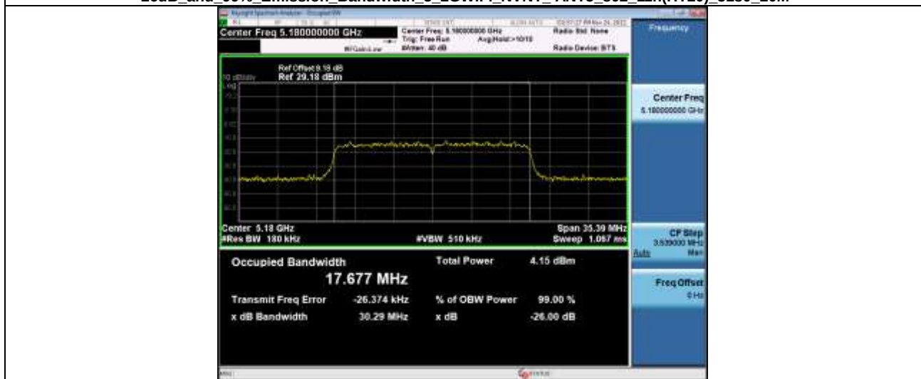
-26dB and 99% Emission Bandwidth 5_2GWiFi_NVNT_ANT5_802_11n(HT20)_5180_20M
