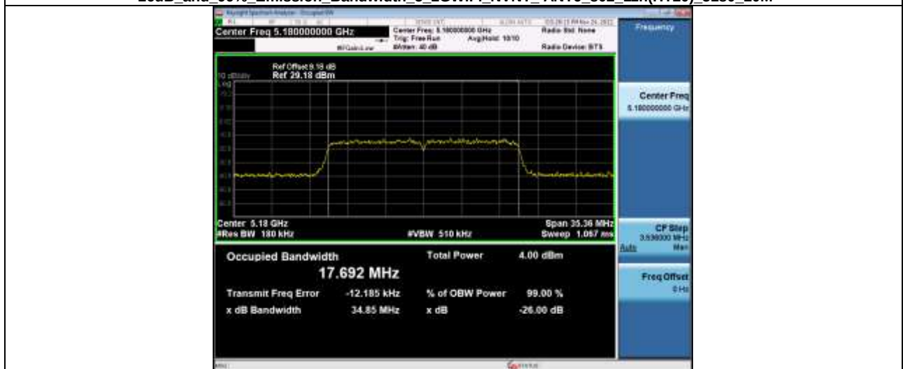
-26dB and 99% Emission Bandwidth 5_2GWiFi NVNT_ANT6_802_11n(HT20)_5180_20M
