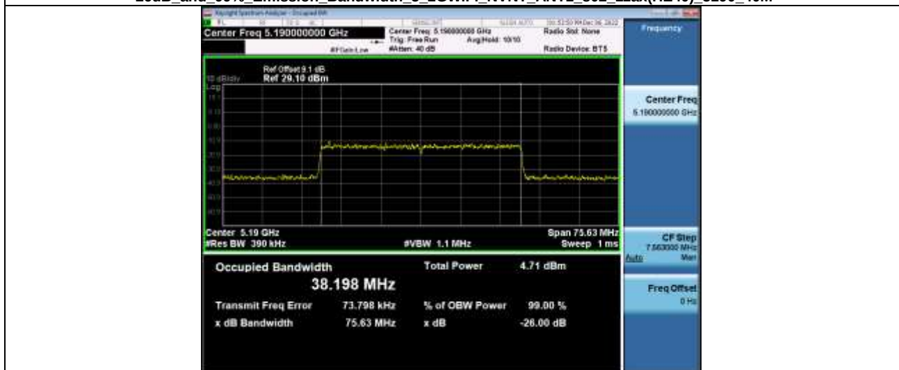
-26dB and 99% Emission Bandwidth 5_2GWiFi_NVNT_ANT1_802_11ax(HE40)_5190_40M
