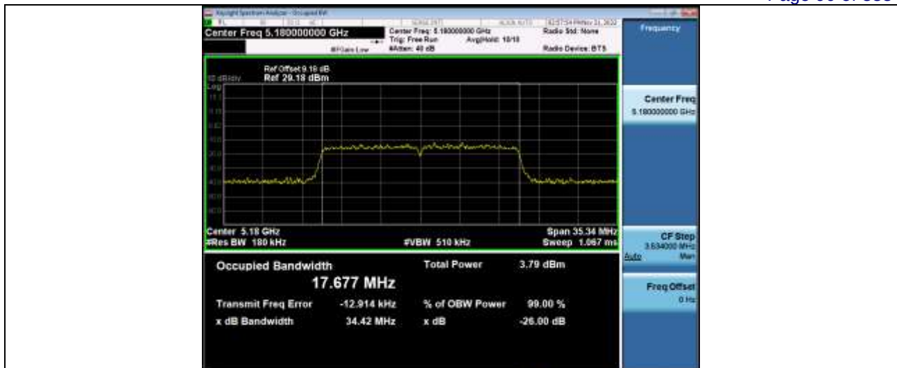
-26dB and 99% Emission Bandwidth 5_2GWiFi_NVNT_ANT1_802_11n(HT20)_5200_20M
