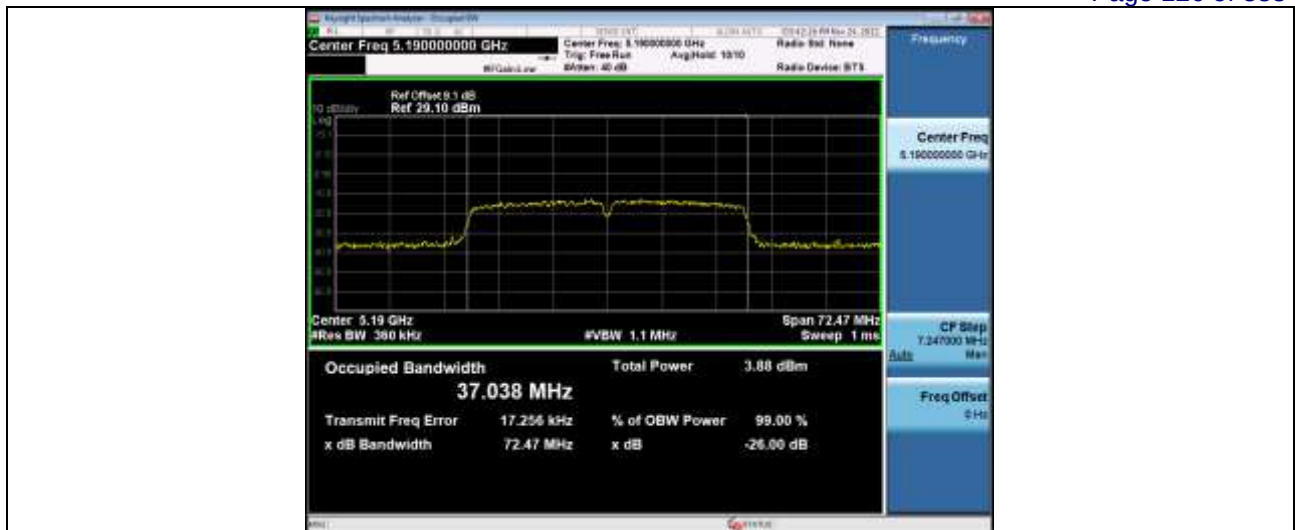
-26dB and 99% Emission Bandwidth 5_2GWiFi_NVNT_ANT6_802_11ac(VHT40)_5230_40M
