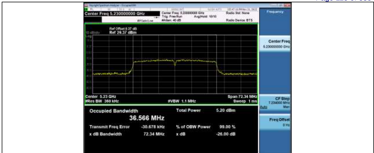
-26dB and 99% Emission Bandwidth 5_2GWiFi_NVNT_ANT4_802_11ac(VHT80)_5210_80M
