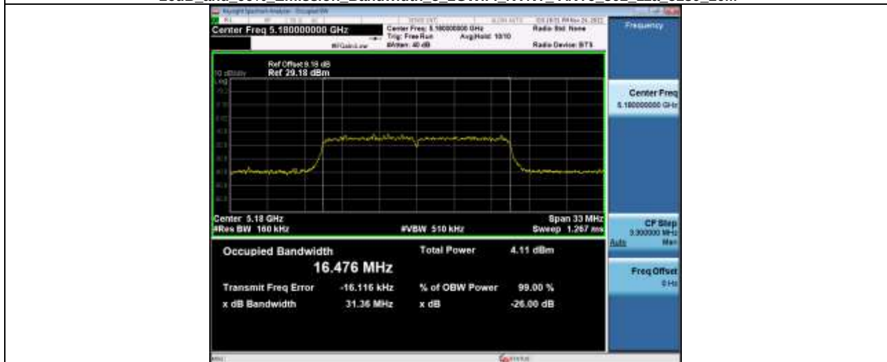
-26dB and 99% Emission Bandwidth 5_2GWiFi_NVNT_ANT6_802_11a_5180_20M
