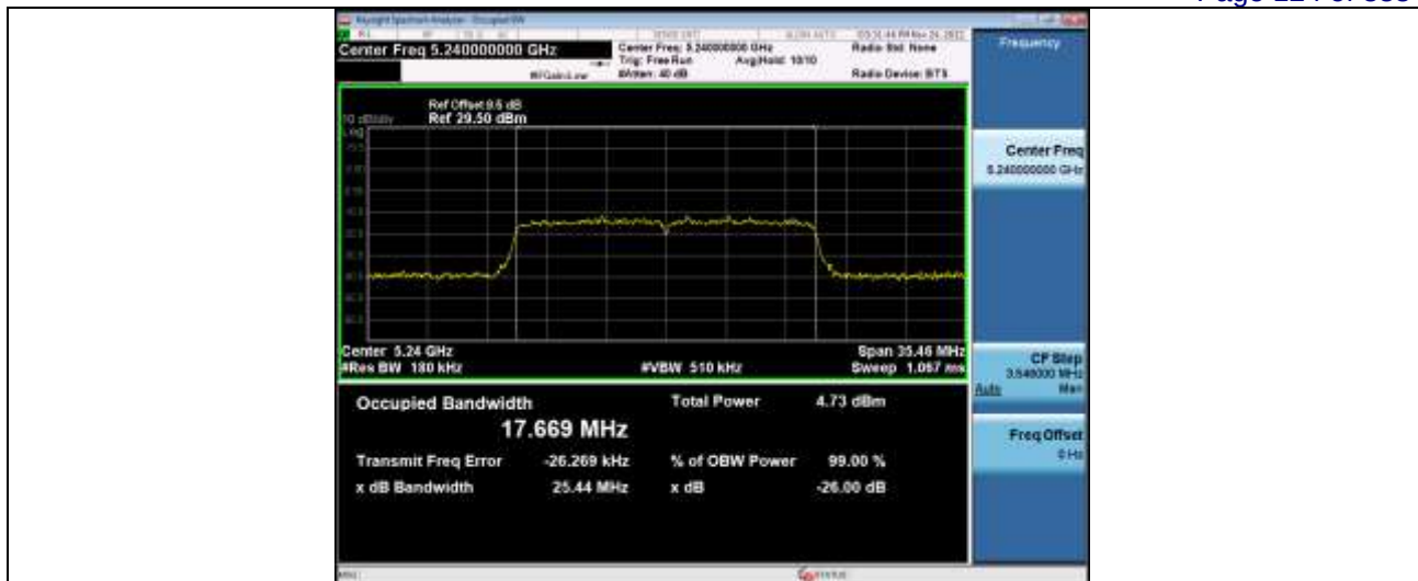
-26dB and 99% Emission Bandwidth 5_2GWiFi_NVNT_ANT6_802_11ac(VHT20)_5180_20M
