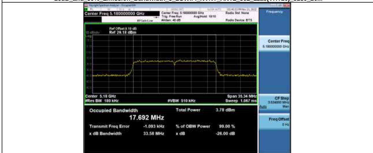
-26dB and 99% Emission Bandwidth 5_2GWiFi_NVNT_ANT2_802_11ac(VHT20)_5180_20M
