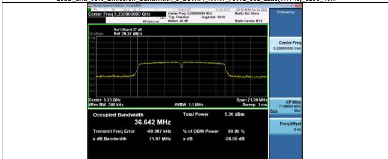
-26dB and 99% Emission Bandwidth 5_2GWiFi_NVNT_ANT2_802_11ac(VHT80)_5210_80M
