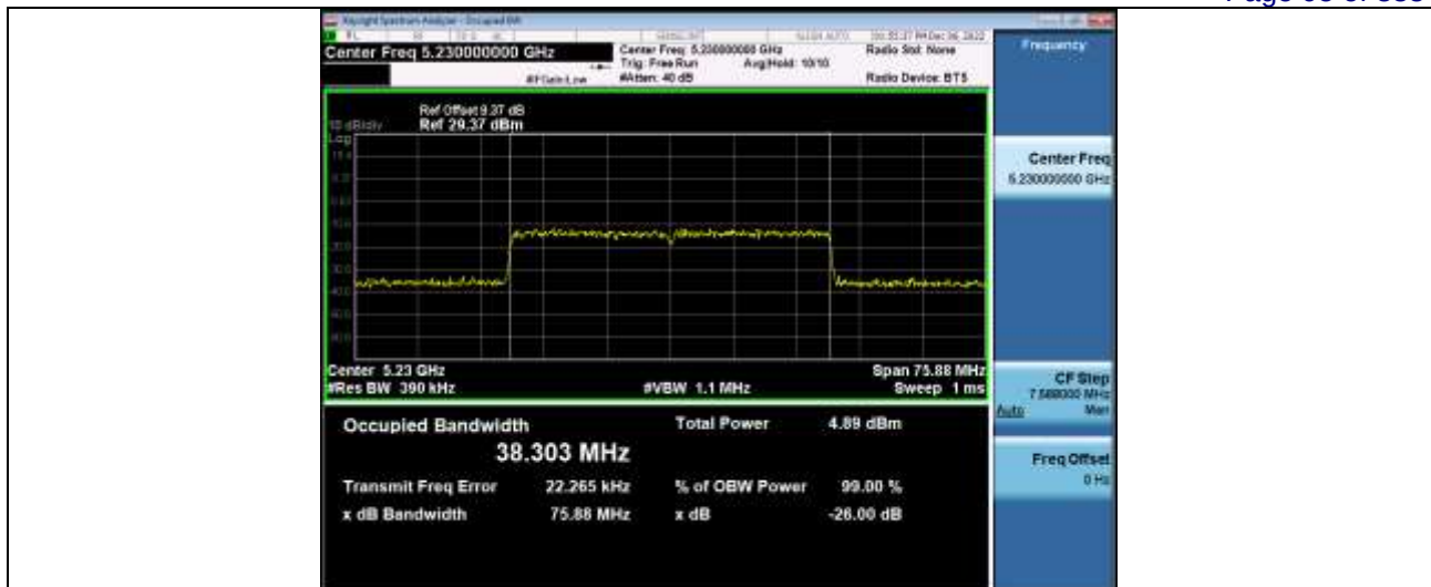
-26dB and 99% Emission Bandwidth 5_2GWiFi_NVNT_ANT1_802_11ax(HE80)_5210_80M
