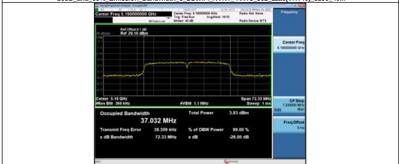
-26dB and 99% Emission Bandwidth 5_2GWiFi_NVNT_ANT5_802_11ac(VHT40)_5230_40M
