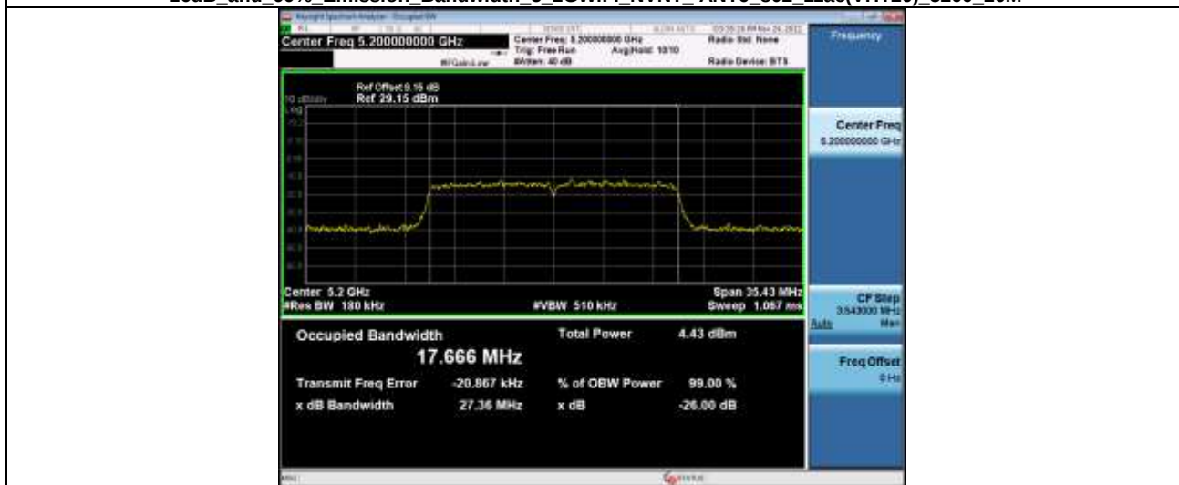
-26dB and 99% Emission Bandwidth 5_2GWiFi_NVNT_ANT6_802_11ac(VHT20)_5240_20M
