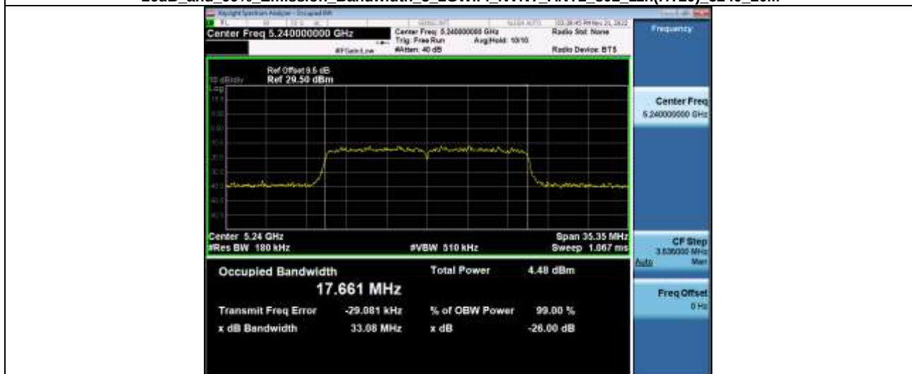
-26dB and 99% Emission Bandwidth 5_2GWiFi_NVNT_ANT2_802_11n(HT20)_5240_20M
