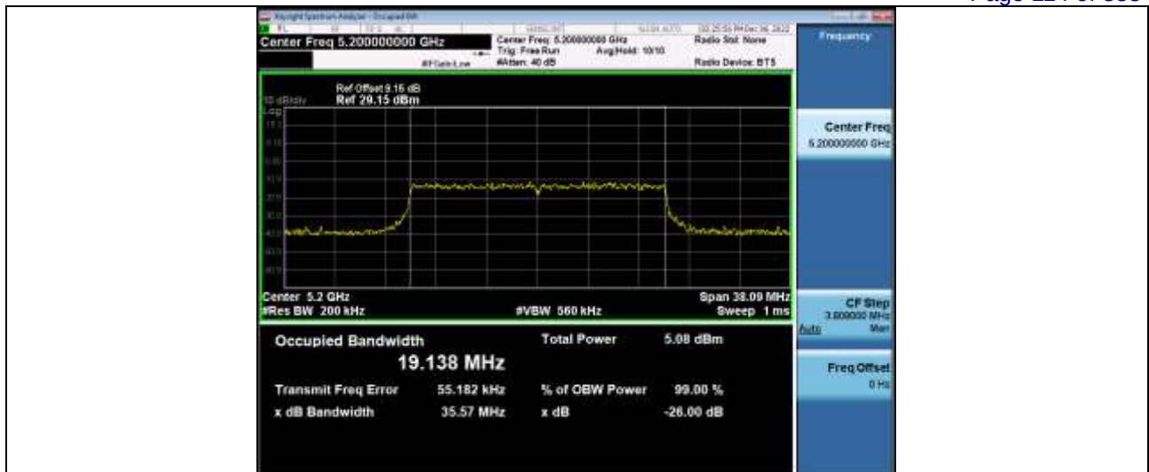
-26dB and 99% Emission Bandwidth 5_2GWiFi_NVNT_ANT4_802_11ax(HE20)_5240_20M
