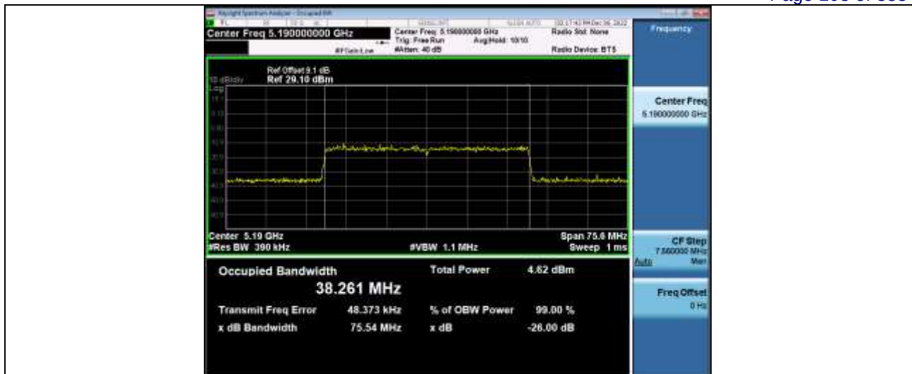
-26dB and 99% Emission Bandwidth 5_2GWiFi_NVNT_ANT3_802_11ax(HE40)_5230_40M
