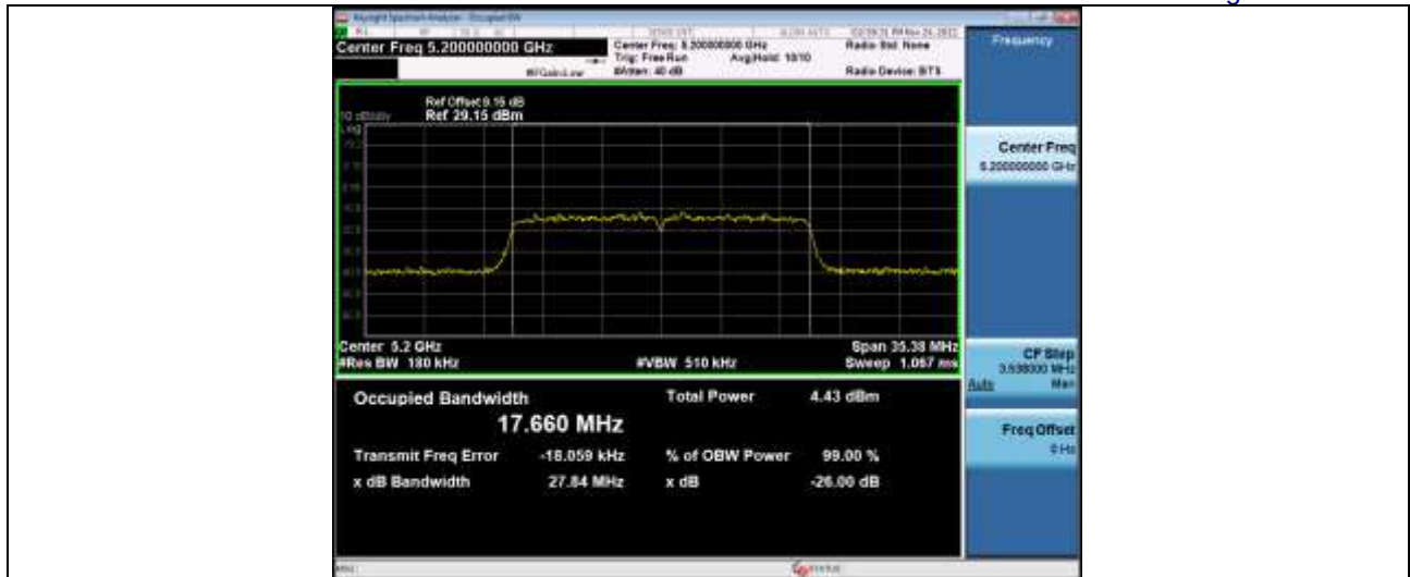
-26dB and 99% Emission Bandwidth 5_2GWiFi_NVNT_ANT5_802_11n(HT20)_5240_20M
