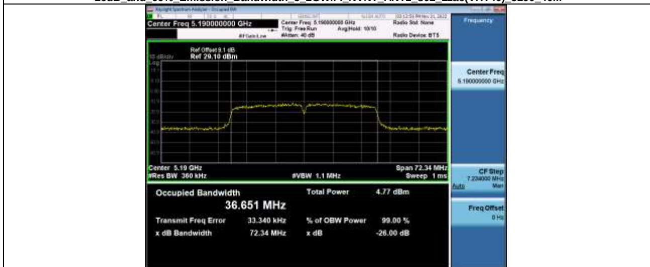
-26dB and 99% Emission Bandwidth 5_2GWiFi_NVNT_ANT1_802_11ac(VHT40)_5190_40M
