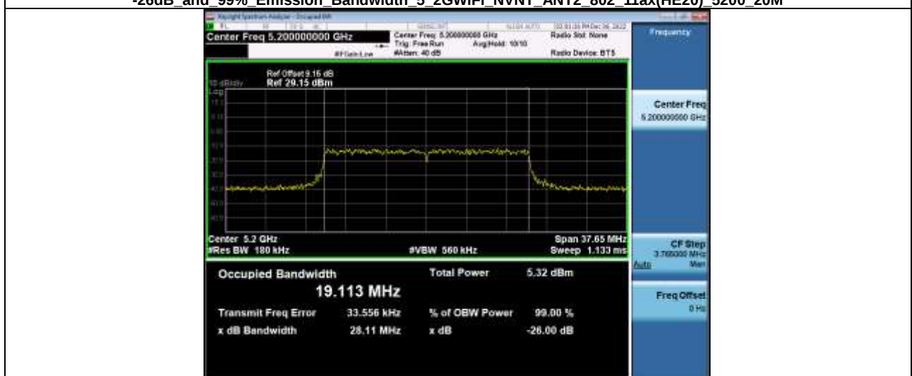
-26dB and 99% Emission Bandwidth 5 2GWiFi NVNT_ANT2_802_11ax(HE20)_5240_20M
