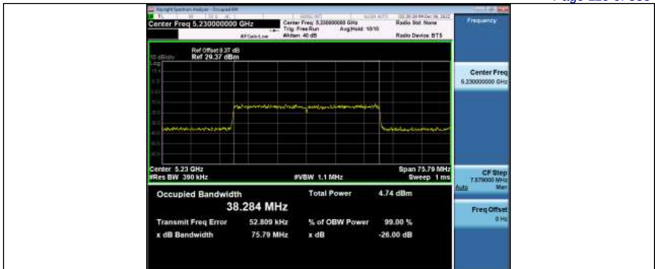
-26dB and 99% Emission Bandwidth 5_2GWiFi_NVNT_ANT4_802_11ax(HE80)_5210_80M
