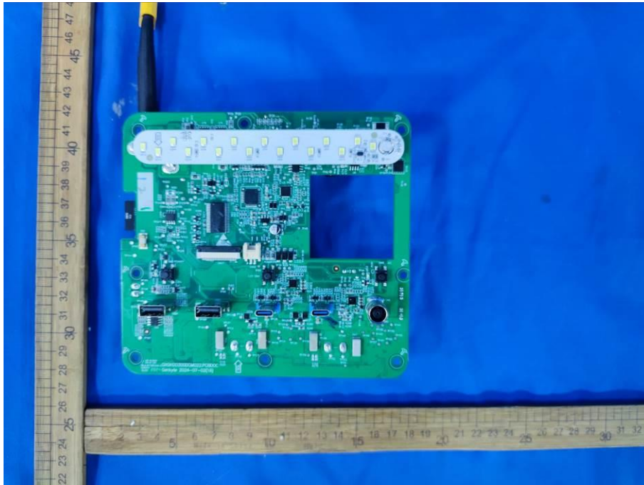
Figure 6. PCB of Main board & BMS board
