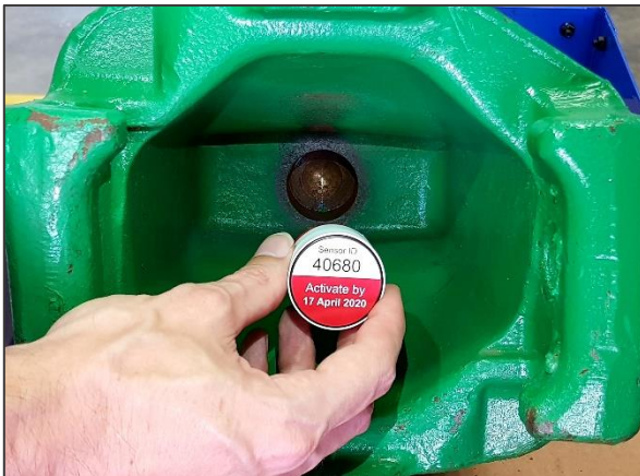
Picture 2. GET Sensor ready to be inserted into the recess of a digger tooth.
