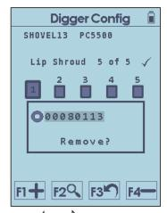
8. Use <sup>⟨</sup> and <sup>⟩</sup> to navigate. 'F4' then <sup>⊚</sup> to deactivate a Sensor
