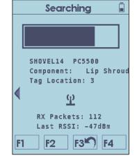
6. Use the search bar to detect and locate the missing GET component.
