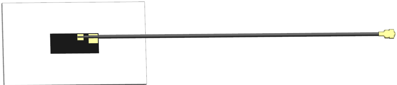
FIGURE4.1.1 ANTENNA LOADED WITH PC/ABS BLOCK OF 1.5MM THICKNESS
