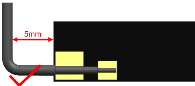
FIGURE 5.2.1 RECOMMENDED CABLE BENDING RANGE
