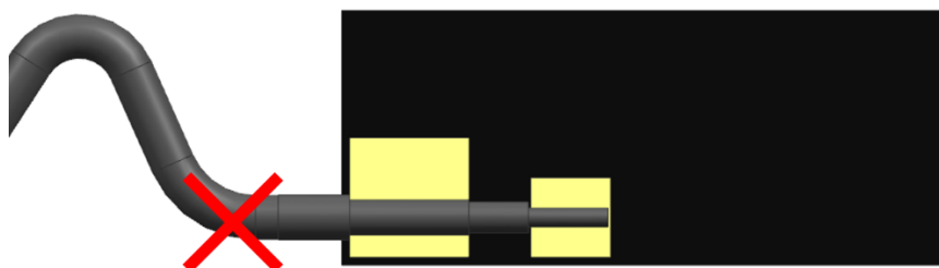
FIGURE 5.2.3 MULTIPLE BENDING OF CABLES IS NOT RECOMMENDED
